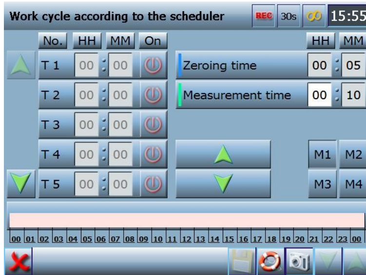
Drawing 47 Work cycle according to the scheduler screen – scheduled measurements mode
