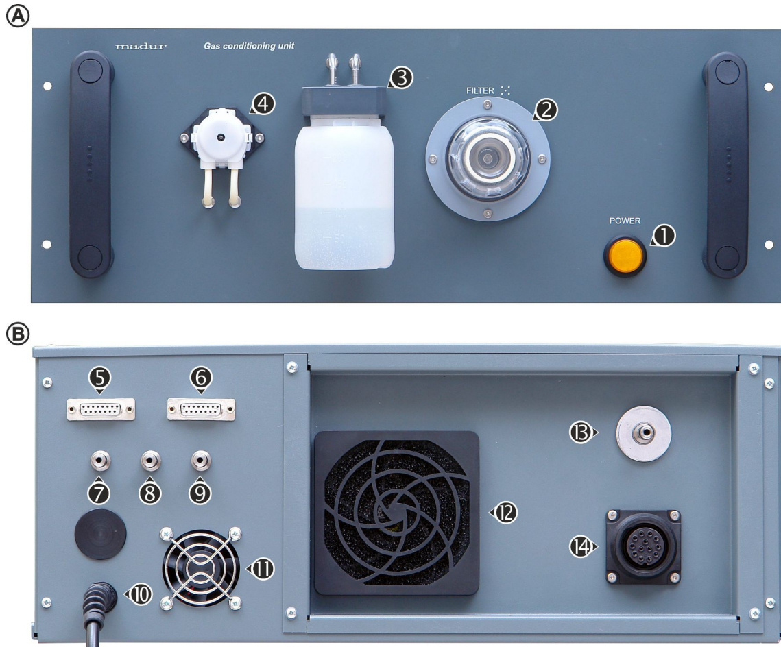
Drawing 3 Gas conditioning unit. A – front view, B – rear view.
